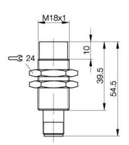
**Inductive Sensors** BES 515-360-E5-T-S 4 M18x1 x 54.5 normally-open Sn=8mm unshielded
